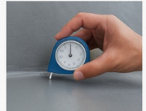
During Application Measure wet film thickness
